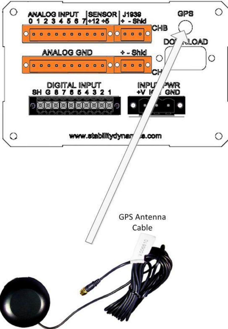
Fig. 12 – GPS Antenna connection to Madass Main Unit
