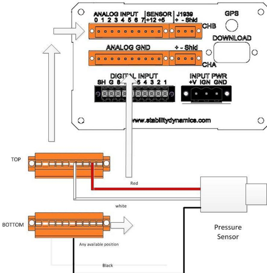
Fig 15. – Pressure Sensor Connection to Madass Main Unit
