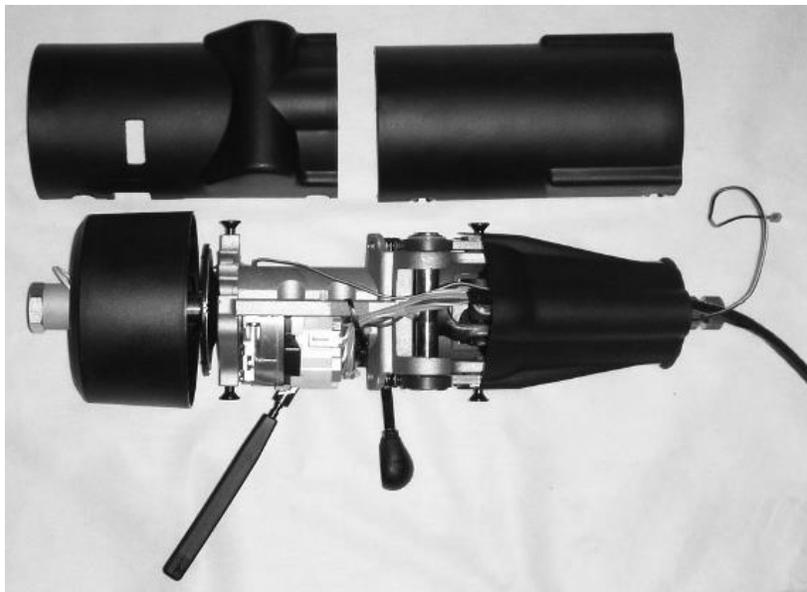
5. Remove the lower plastic housing by pulling the upper tabs off of the mounting pin and then pulling the housing down onto the lower steering column.
