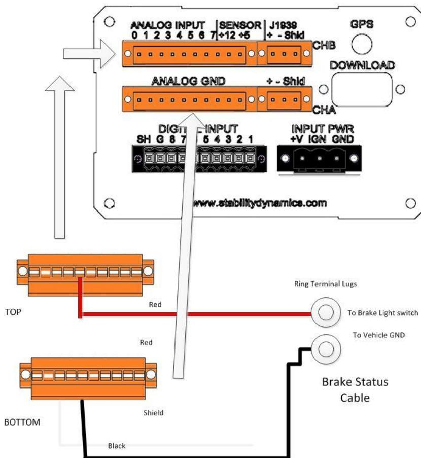
Fig. 14 – Brake Status Indicator connection to Madass Main Unit
