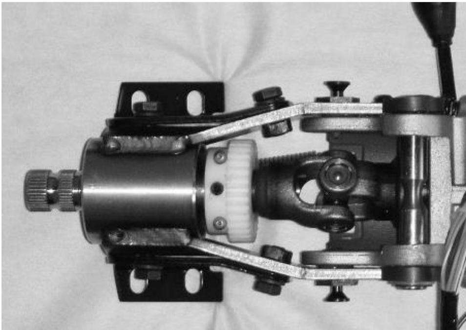
9. Tighten the two bolts which hold the split gear together using the 3/32" Allen key. Be sure to tighten them alternately and evenly to ensure that the split between the two halves of the gear is even on both sides of the shaft. Do not overtighten the bolts. They should only be tightened so the gaps between the two shafts are similar in size to the gaps between the other teeth on the gear.
