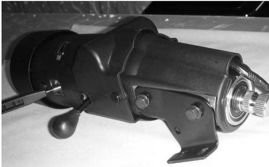
4. Remove both halves of the upper plastic housing by pulling them outwards from the steering shaft off of the four mounting pins (it may take a bit of jostling to remove the housing from the upper pins, but the steering wheel does not need to be removed).
