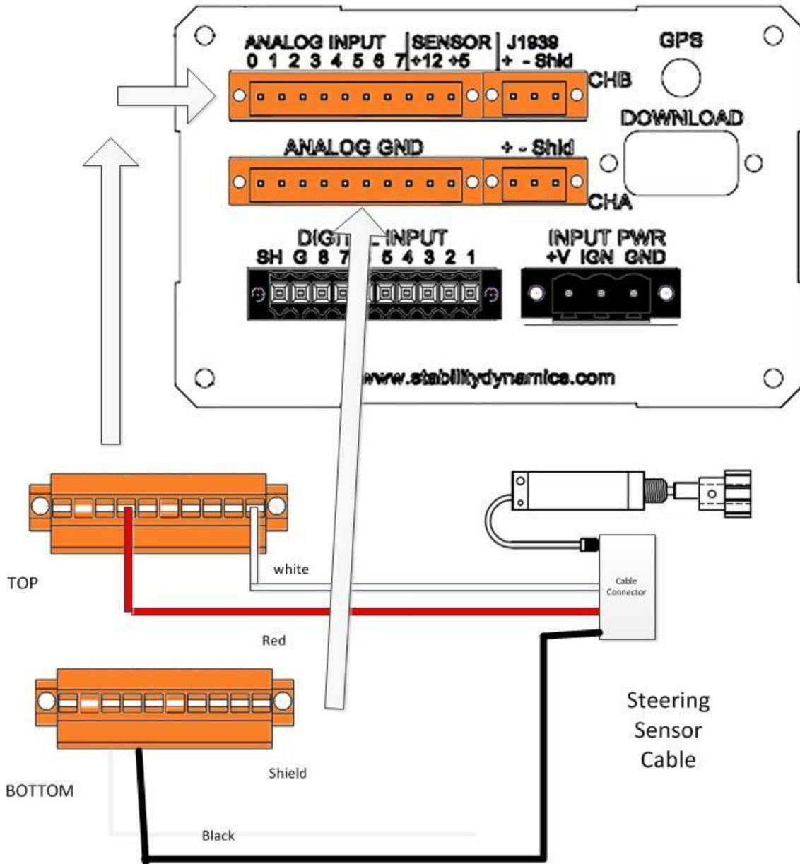
Fig. 13 – Steering Sensor connection to Madass Main Unit
