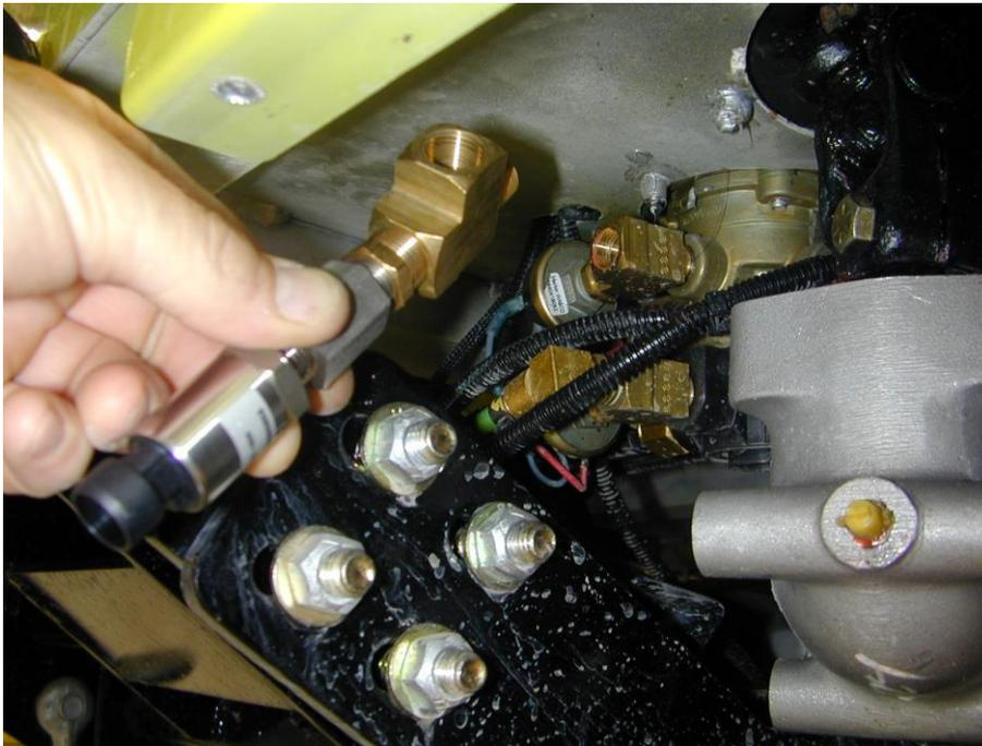
Fig. B1 - Pressure Sensor attached to T-junction manifold
