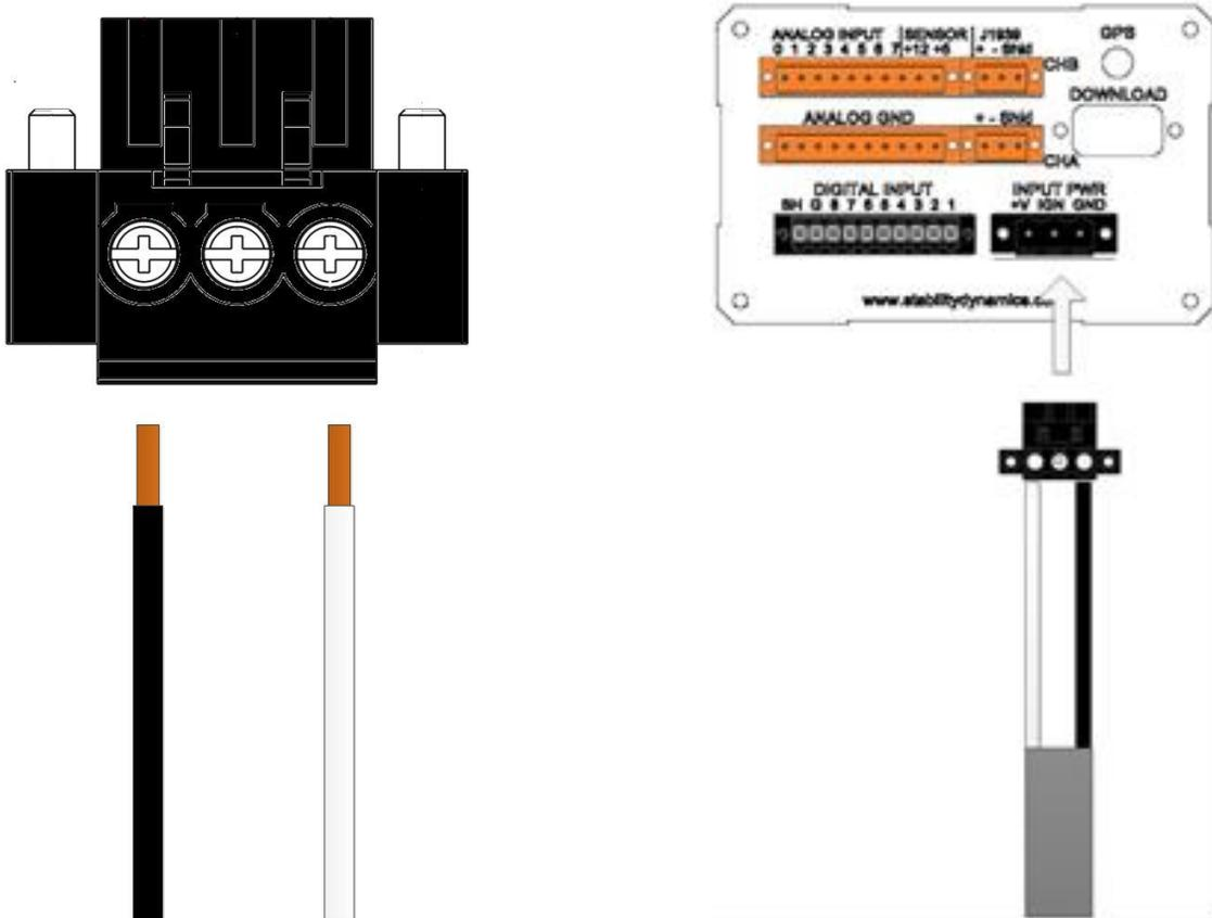
Fig. 3 – MADASS Main unit power connection
