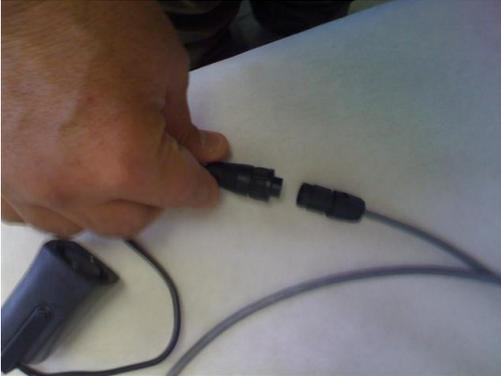
Fig 8- LG Alert Siren connected to Madass Adapter cable
