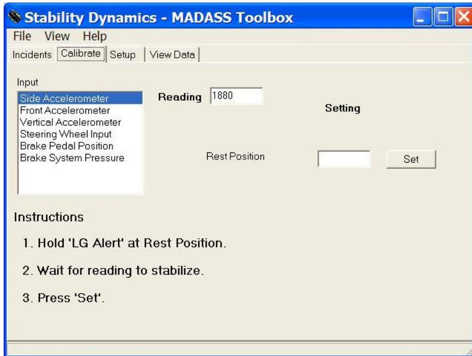
Fig.18 – Sensor Calibration Screen
