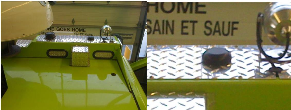
Fig. 11 – Typical GPS Antenna mounted on fiberglass / metal type roof
