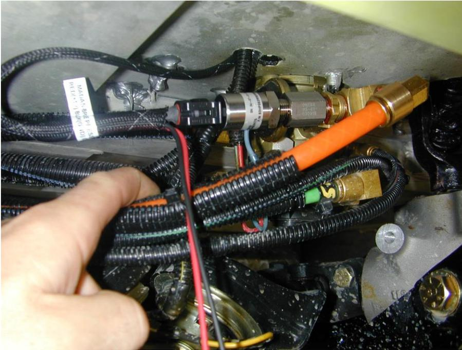
Fig. B2 - Brake Pressure Sensor installed to braking valve air output line, and sensor wiring harness connected to sensor
