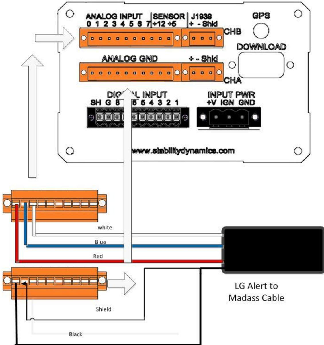
Fig 9 – LG Alert to Madass Main unit wiring
