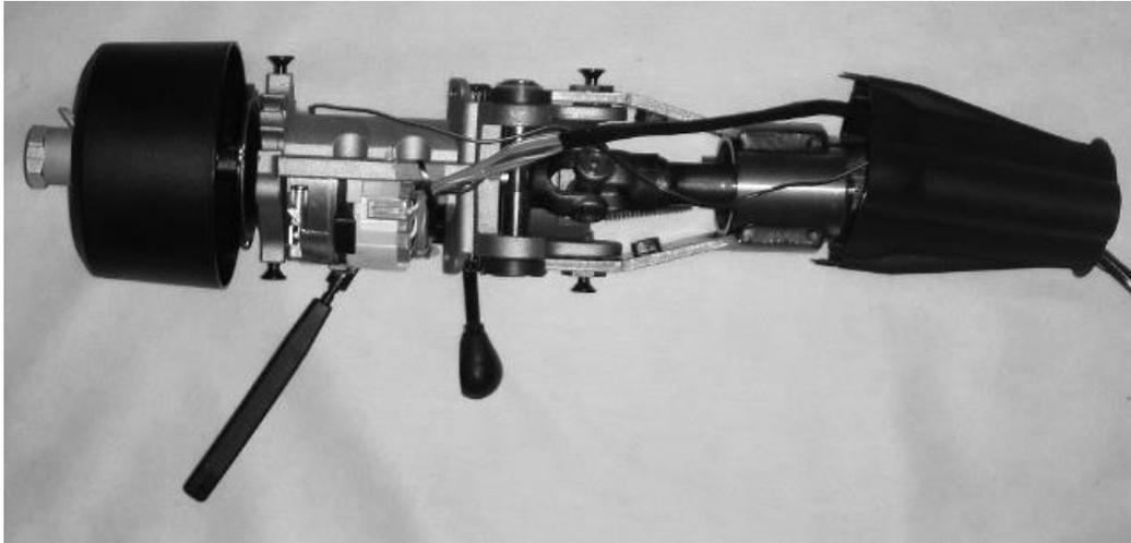
6. Place the steering column back between the brackets and tighten the bolts. This will allow for ease of installation by supporting the column while the remaining steps are completed.
