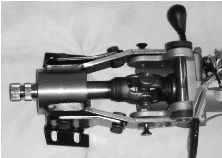
7. Place the lower half of the split gear (the side without the set screw) onto the shaft. It should be placed on the back side of the shaft, with the hub towards the bottom bearing, and as close to the weld at the universal joint as possible.
