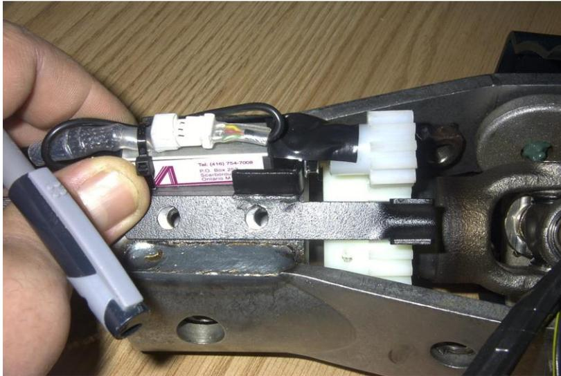
13. Mark the centre of the two holes in the potentiometer mounting bracket.
