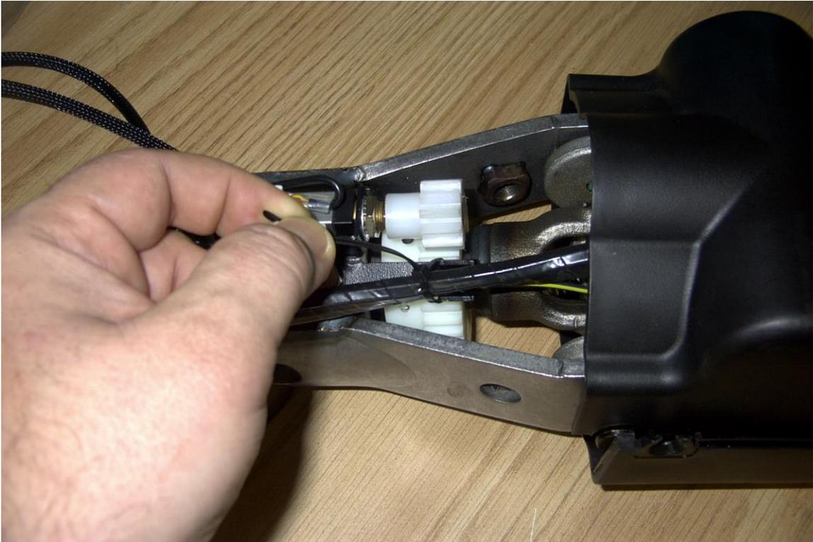
18. Snip the ends of the cable ties using the wire snippers.
