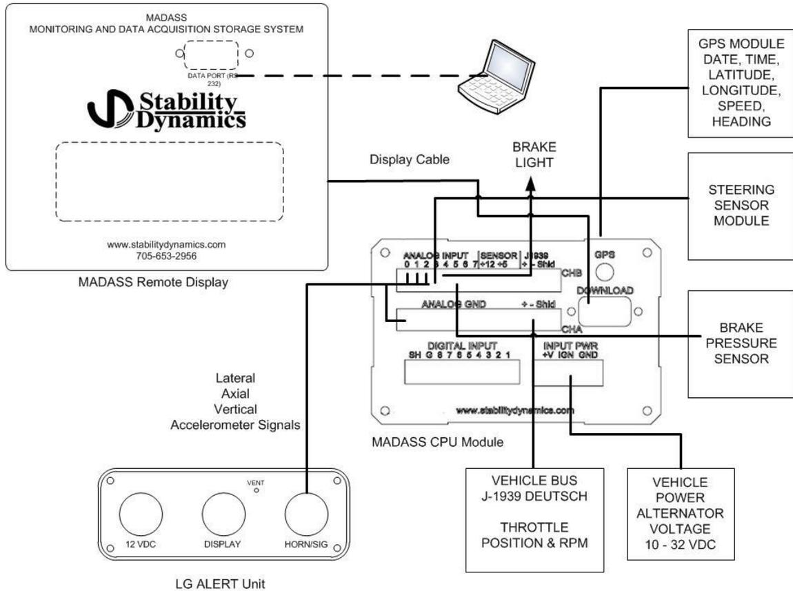
Fig. 1 – MADASS System Block Diagram
